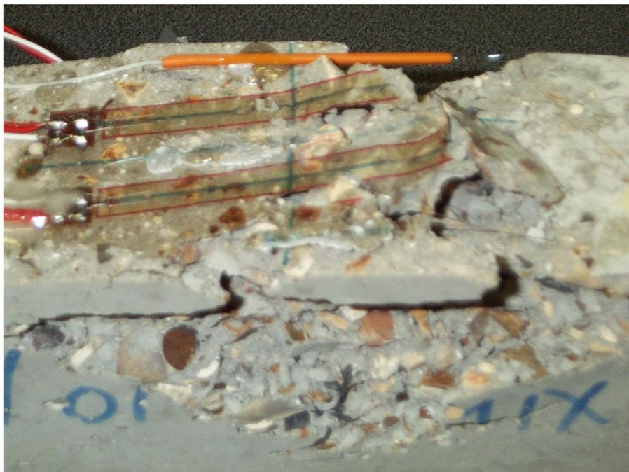
Figure 2. Strain gauges and optical fibre sensors on failed concrete specimens.
